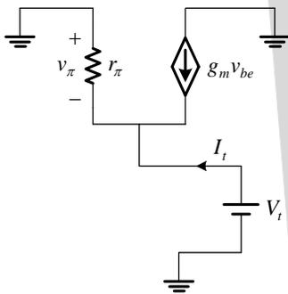
$$\begin{aligned} I &= -\left(g_m v_{\pi} + \frac{v_{\pi}}{r_{\pi}}\right) \\ &= -\left(g_m + \frac{1}{r_{\pi}}\right) \cdot (-V_t) \\ \Rightarrow R_{eq} &= \frac{V_t}{I_t} = \frac{1}{g_m + \frac{1}{r_{\pi}}} = \frac{r_{\pi}}{1 + g_m r_{\pi}} \end{aligned}$$
